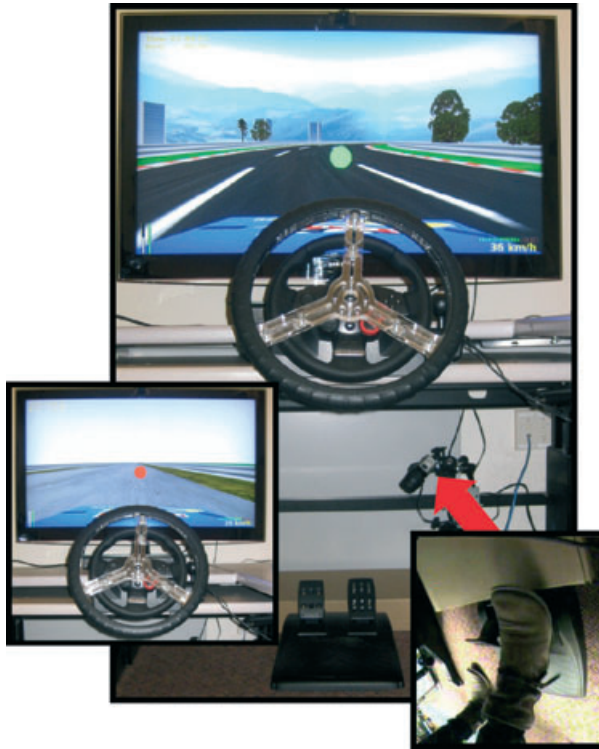
Fig. 1. Simulator layout and experimental setup. The screen shows a typical driver view in the complex condition; the left inset shows a typical view in the simple condition. The right inset shows a sample frame of the camera used for initial foot motion detection.
